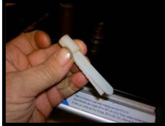
Push the entire assembly into the stopper end with the 3/4" tennon. The wedge and tone board are tapered and will form a tight fit in the stopper. It helps to put the tone board in first sometimes, and push it in further than normal. Then set the wedge in place and pull the toneboard out to for a tight fit.
