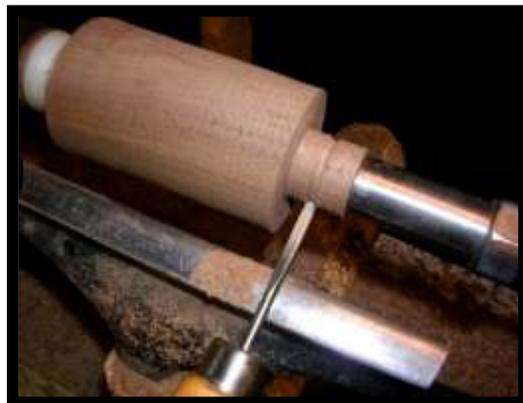
Now that we have the tennon turned, it is time to turn the stopper to the desired shape. I use a pair of calipers to get the diameter of the barrel...
