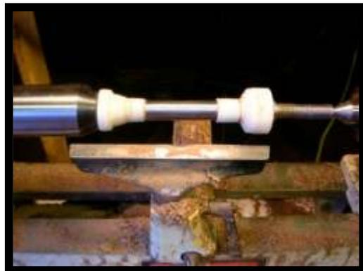
Once I have turned my blank to round, and trued up the ends, I take a measurement with my tone board. The tone board will fit inside the barrel, so you want to keep your barrel at least 3 inches long. Any shorter and the tone board will stick out the end
