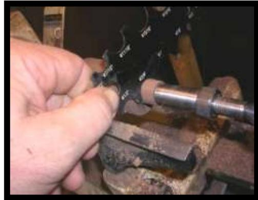
If you do not have a spindle gauge, you can make one by drilling a scrap blank to  $\frac{3}{4}$ " and then cutting it in half. Use it to check the diameter of your tennon.
