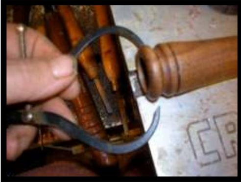
and then use that measurement when turning the stopper. This ensures an even flow from barrel to stopper and makes your call look aesthetically pleasing.
