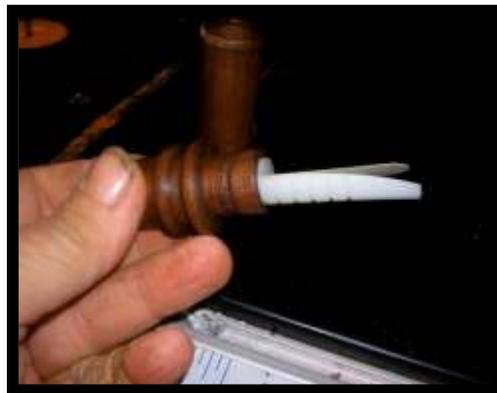
Next, put the large O rings on the tenons and the small O ring on the tone board. I usually use two O rings on the end that goes in the barrel, and do not use one on the expansion tube end. I take care to turn that tenon to a very snug fit.
