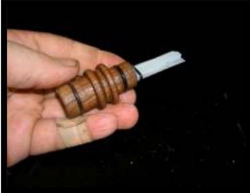
Slide the end of the stopper with the reed into the barrel. The O ring will provide a snug fit.
