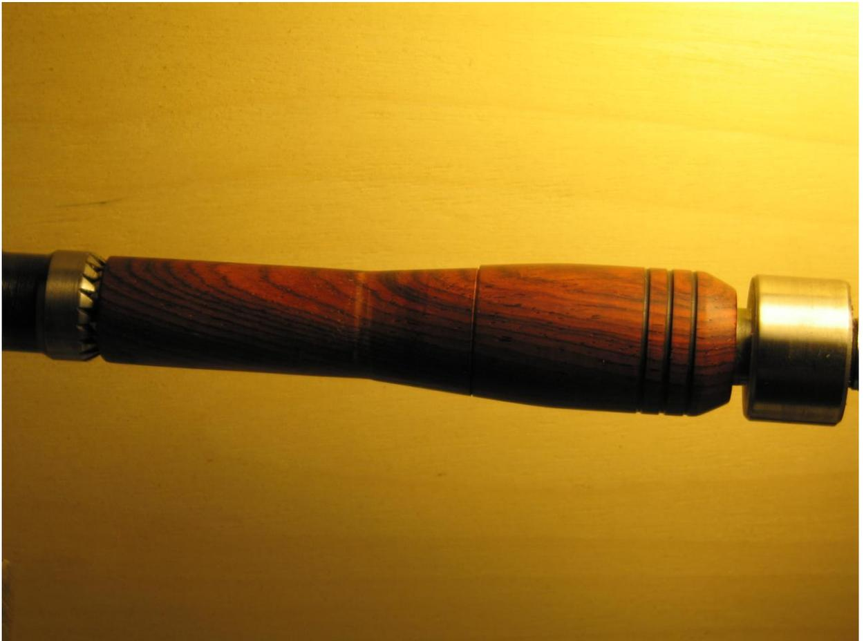
8. Remove the insert from the lathe centers and retain the live center in the tail stock. Remove the drive center from the headstock and replace it with a 3/4 inch collet chuck.
