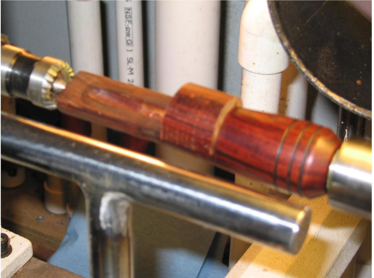
28. With the insert mounted in the lathe turn the wedge block to the taper that matches the existing taper on the remainder of the insert.
