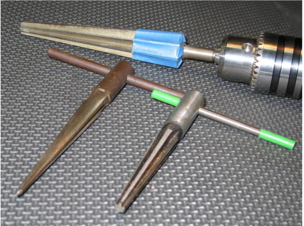
The top reamer in the picture is the reamer I used to ream the taper in the exhaust end of the barrel. The blue tape marks the depth. The reamer with the green handle is the modified handyman's reamer that is used to work the exhaust hole only. The remaining reamer is an unmodified handyman's reamer.
