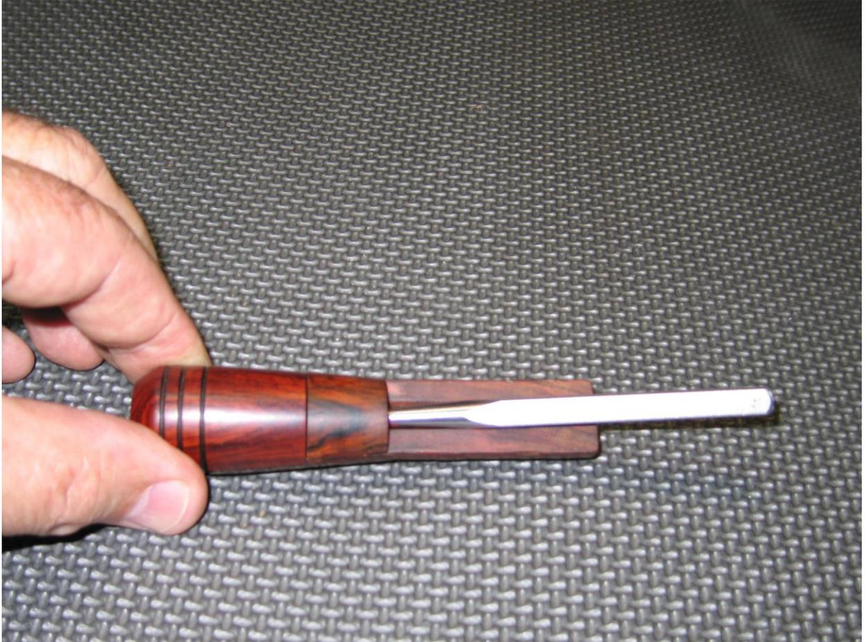
31. We now have a finished insert and wedge that should fit into our barrel. Slip a metal reed under the wedge and check the fit of the insert, wedge and barrel. Adjust the fit as necessary. The wedge should fit into in the barrel taper by a least  $1/2$  to  $2/3$ rds of its overall length. I prefer  $2/3$ rds.
