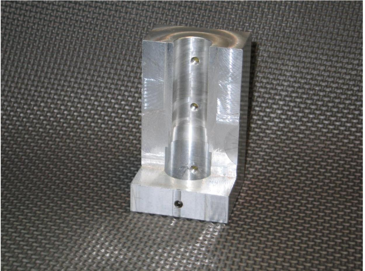
17. Place the insert in the tone board cutting fixture. The fixture has screws to adjust the position of the insert in the fixture. The insert should set level in the fixture when the screws are properly adjusted.
